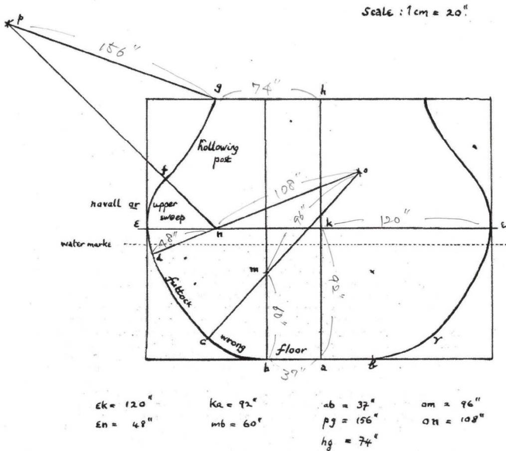
Fig. 1 Harriot's midship mould or bend (f.48) [Reconstruction]
