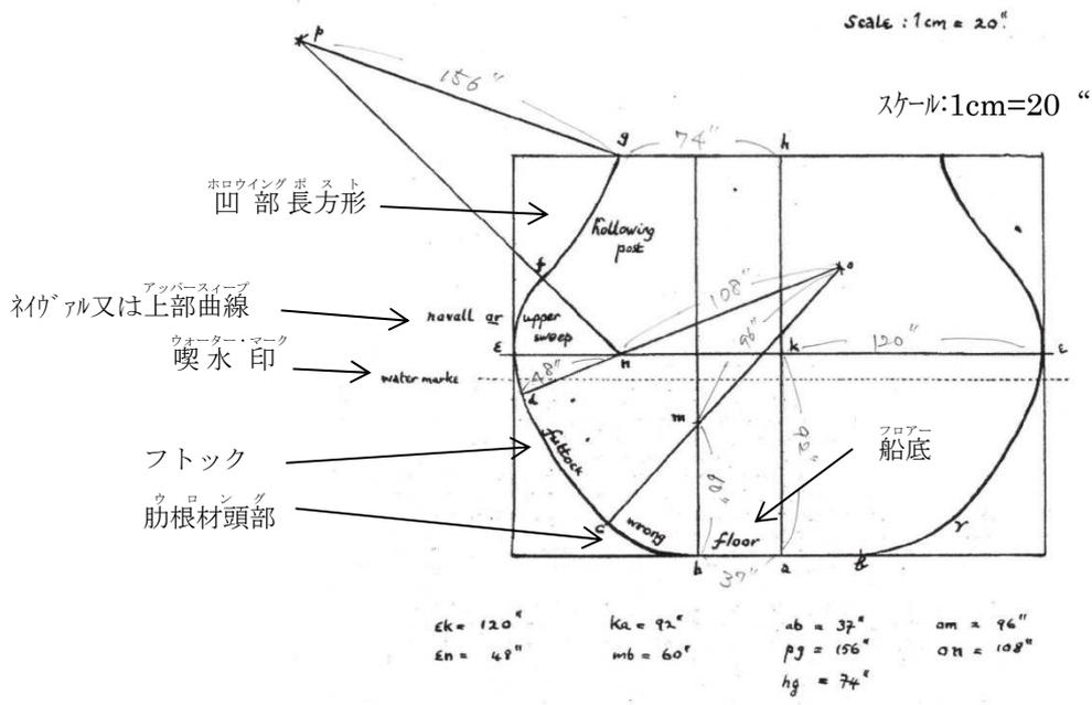
Fig. 1 Herriot's midship mould or bend (f.48) [Reconstruction]
